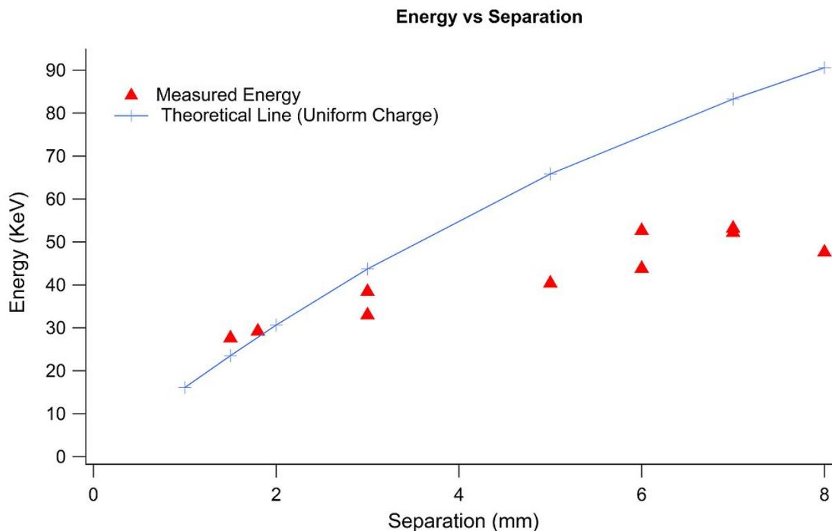
This graph shows the energy of the band system with varying target separation distance. This data was taken from various runs on Caroline, and includes data points from a variety of loop widths. It can be seen that the energy does not increase with distance as rapidly as a uniform charge distribution would predict.
