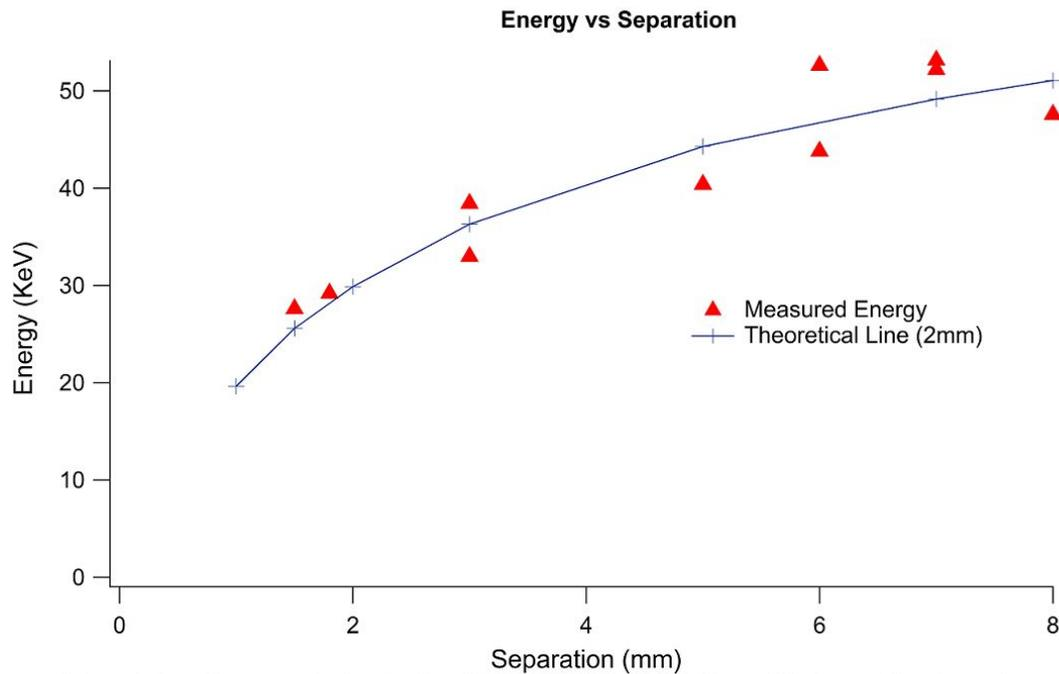
This graph shows the energy of the band system with varying target separation distance. This data was taken from various runs on Caroline, and includes data points from a variety of loop widths. These measurements fit the theoretical curve of a 2mm long rectangular charged region. (2mm was determined to be the best fit through least squares methods).
